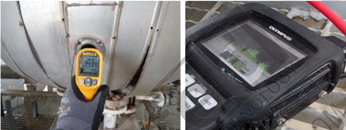
Figure 1: 5 MHz probe, producing an insufficient signal-to-noise ratio.
